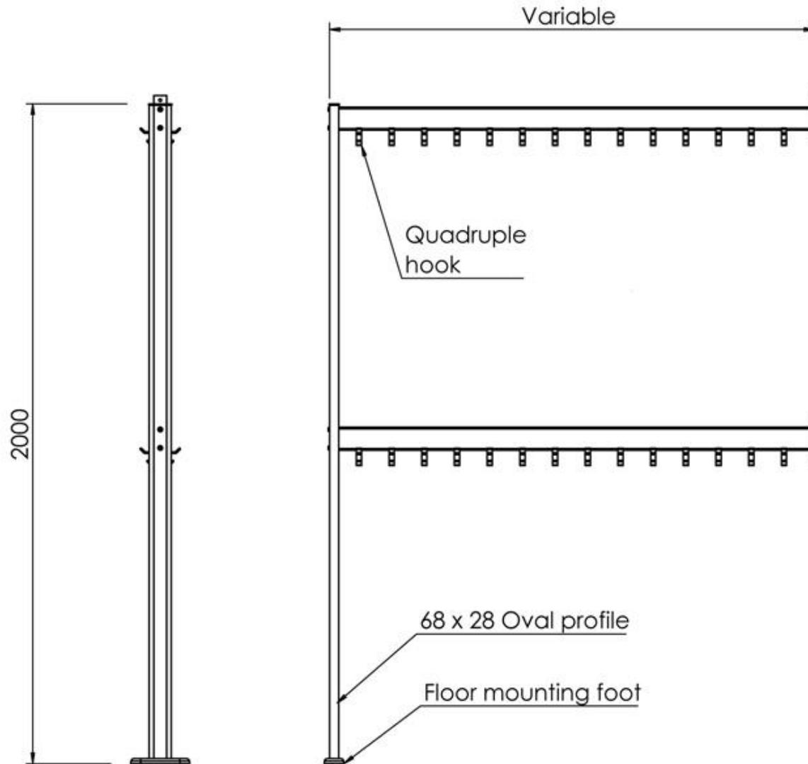
Individual rail lengths up to 2500mm. For longer rail sections additional support legs are required.
