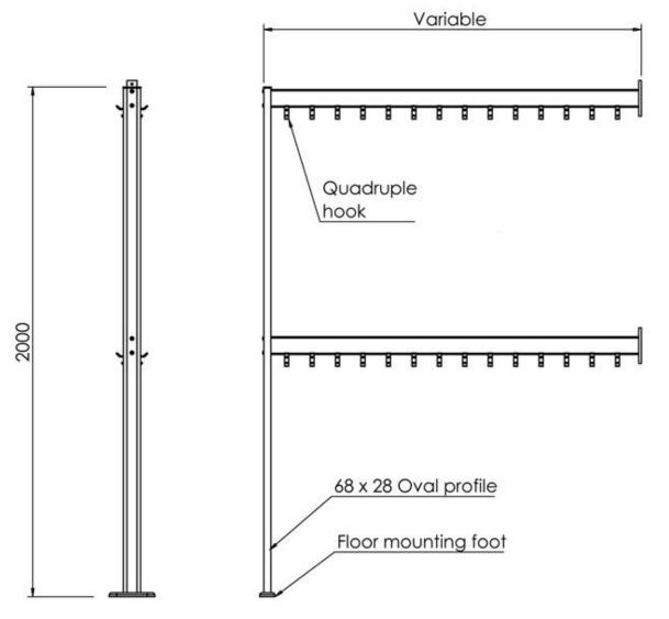
Individual rail lengths up to 2500mm. For longer rail sections additional support legs are required.
