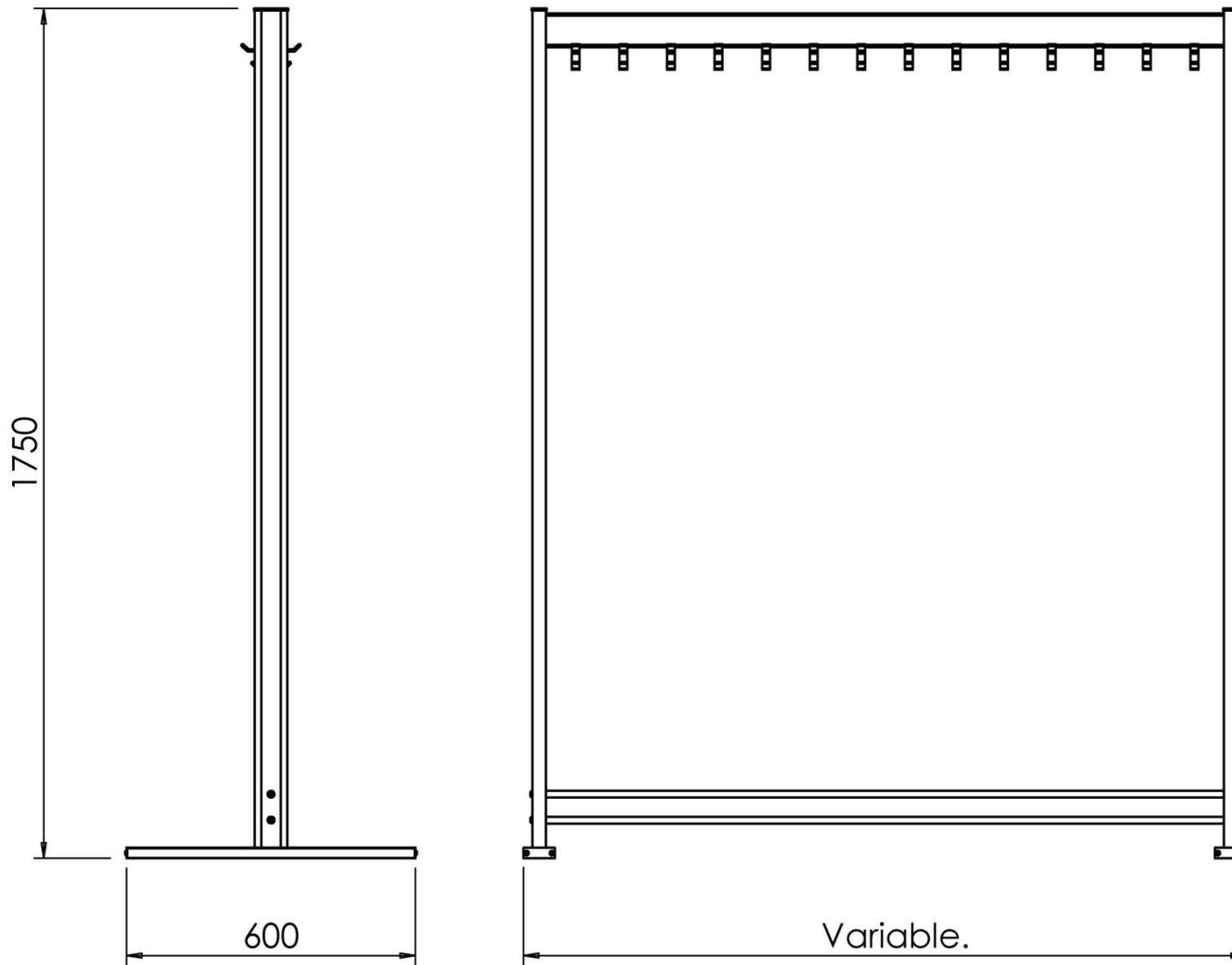
Rail lengths variable up to 2500mm.
