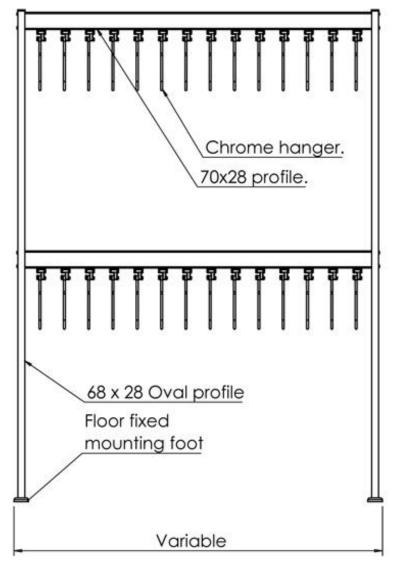
Individual rail lengths up to 2500mm. For longer rail sections additional support legs are required.
