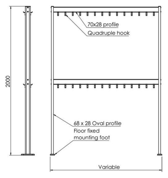
Individual rail lengths up to 2500mm. For longer rail sections additional support legs are required.
