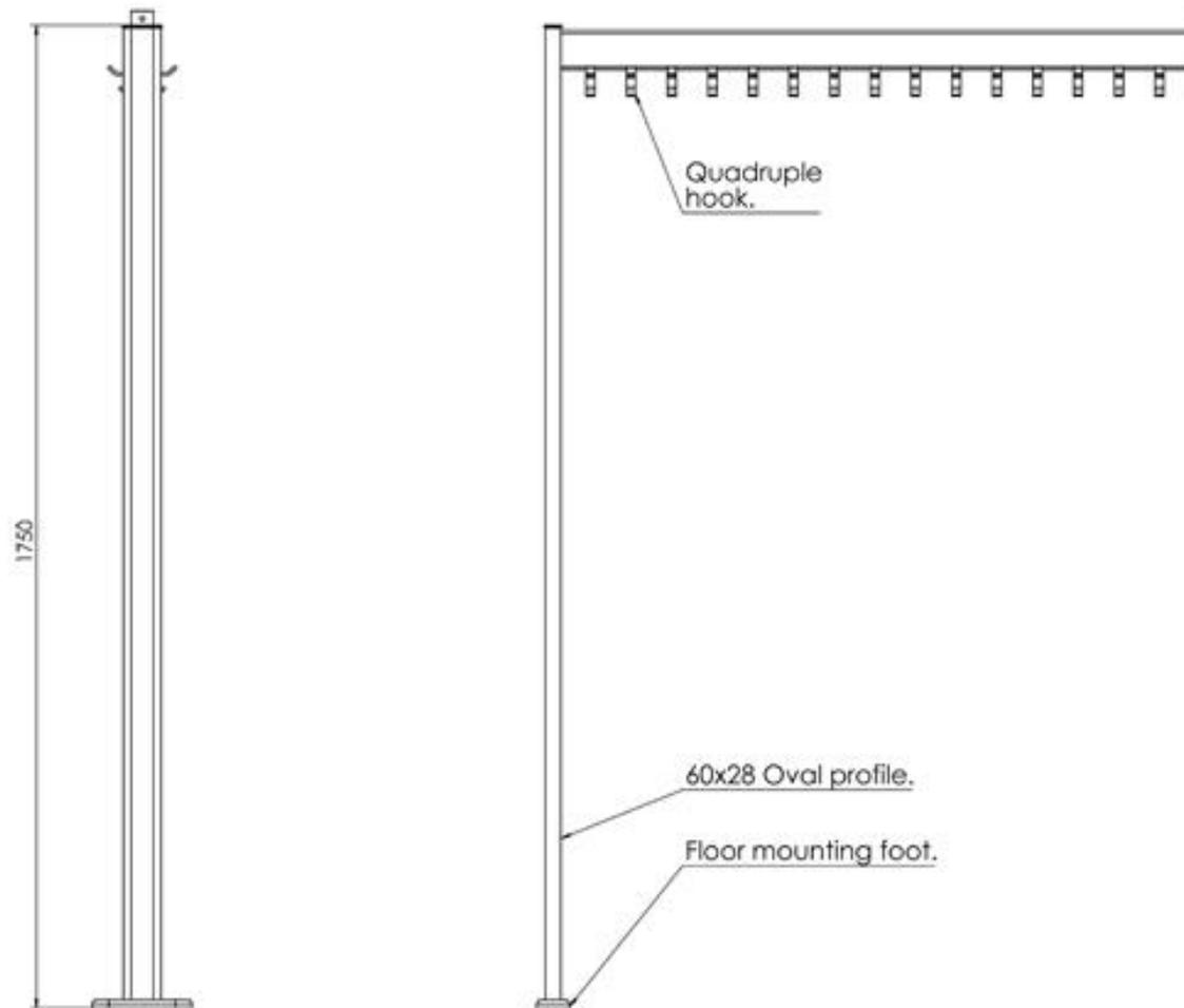
Individual rail lengths up to 2500mm. For longer rail sections additional support legs are required.
