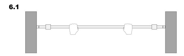
Person 2 pushes the wall bearing outer sleeves outwards - all the way to the wall. TIP: If you turn the outer sleeves so that the fixing screws point backwards, they will no longer be visible from the front later.
