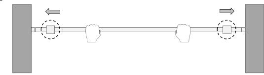
Person 2 tightens all 4 fixing screws with the Allen key provided. Then the assembly is complete.
