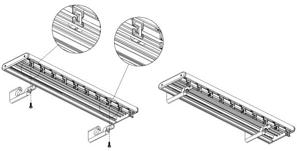
Space out fixing nuts within rail to line up with brackets, then place rail on brackets, fix the rail from below using M8 bolts provided into the fixing nuts (see above). Ensure rail is firmly fixed.
