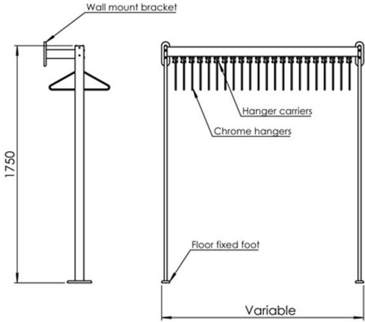
Individual rail lengths up to 2000mm. For longer rail sections additional support legs are required.
