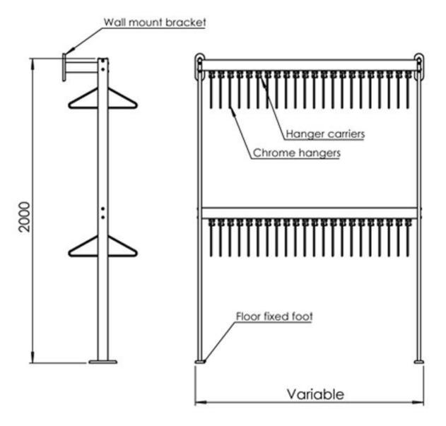
Individual rail lengths up to 2000mm. For longer rail sections additional support legs are required.
